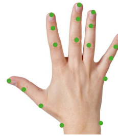
Figure A.1: Our custom marker definition for motion capture during data collection.
